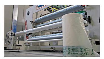
**Eco-Corr® Biodegradable VpCI® Film** – Aliphatic-aromatic co-polyester, VpCI® film. Degrades 100% into carbon dioxide and water once composted. Provides multi-metal corrosion inhibition and eliminates waste. BPI Certified Compostable. Available in formulations up to 40% biobased content.
