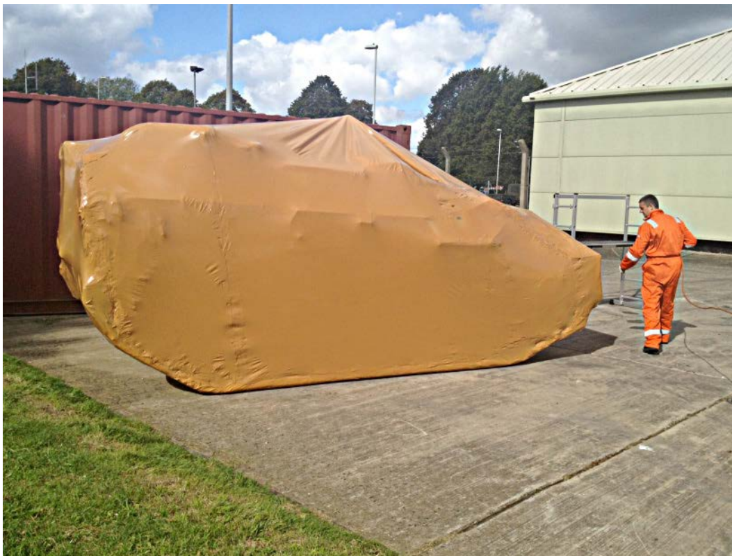
Figure 6: VCI aerosol used to protect Combat Vehicle Reconnaissance (CVR) (5) wheels. VCI additives were also used in the fuel, coolant, engine, gearbox, drive, and brake systems.
