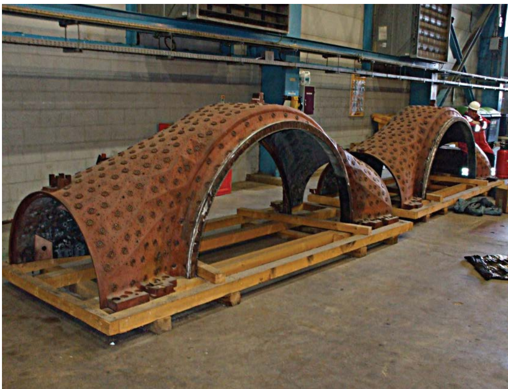
Figure 10: Gas turbine shells, prior to preservation.
