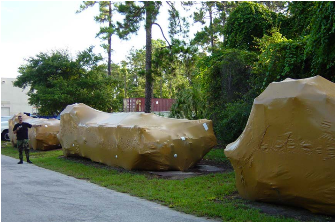
Figure 9: Three United States Air Force Cargo Loaders, preserved with VCI shrink film.
