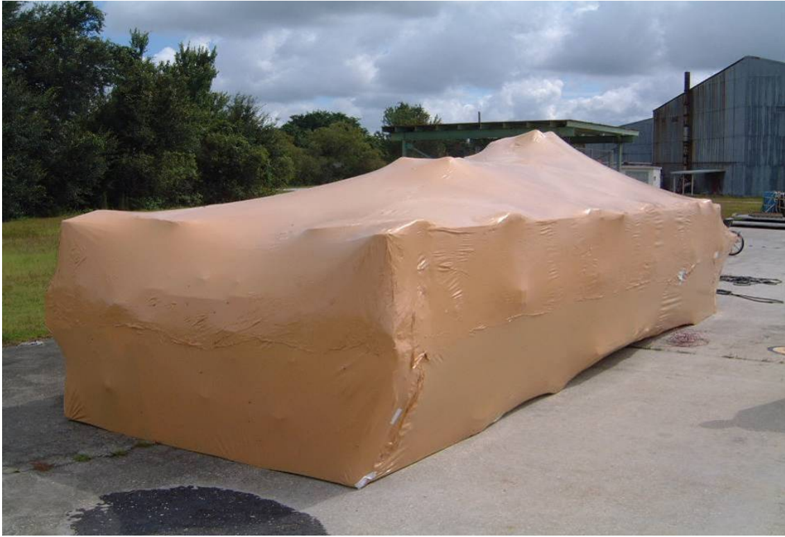
Figure 1: Fully preserved military equipment, after preservation with an integrated VCI system.
