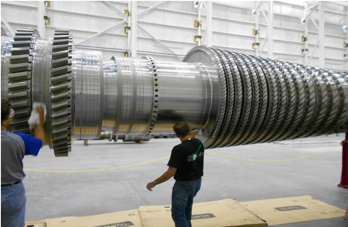
Figure 12: Rotor being cleaned prior to preservation.
