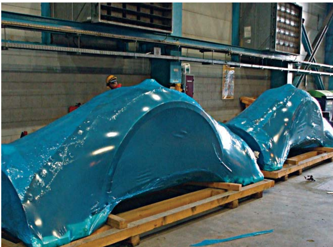
Figure 11: Gas turbine shells, after preservation with VCI shrink film.
