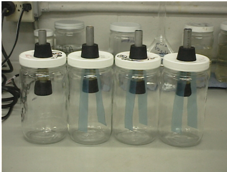
Figure 2: VIA Test Setup, with VCI film.
