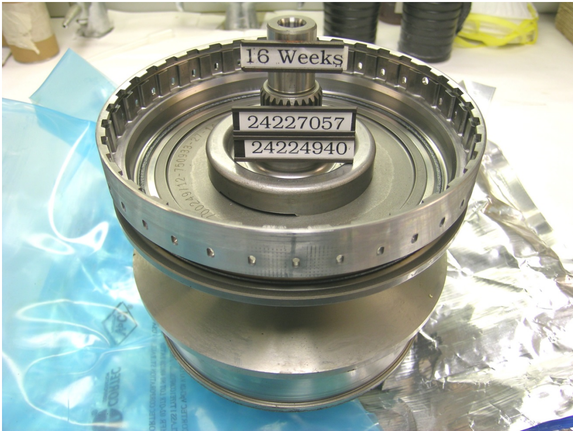
Figure 5: Automotive transmission component, after 16 weeks in modified ASTM (4) D-1748 testing, wrapped in VCI film.
