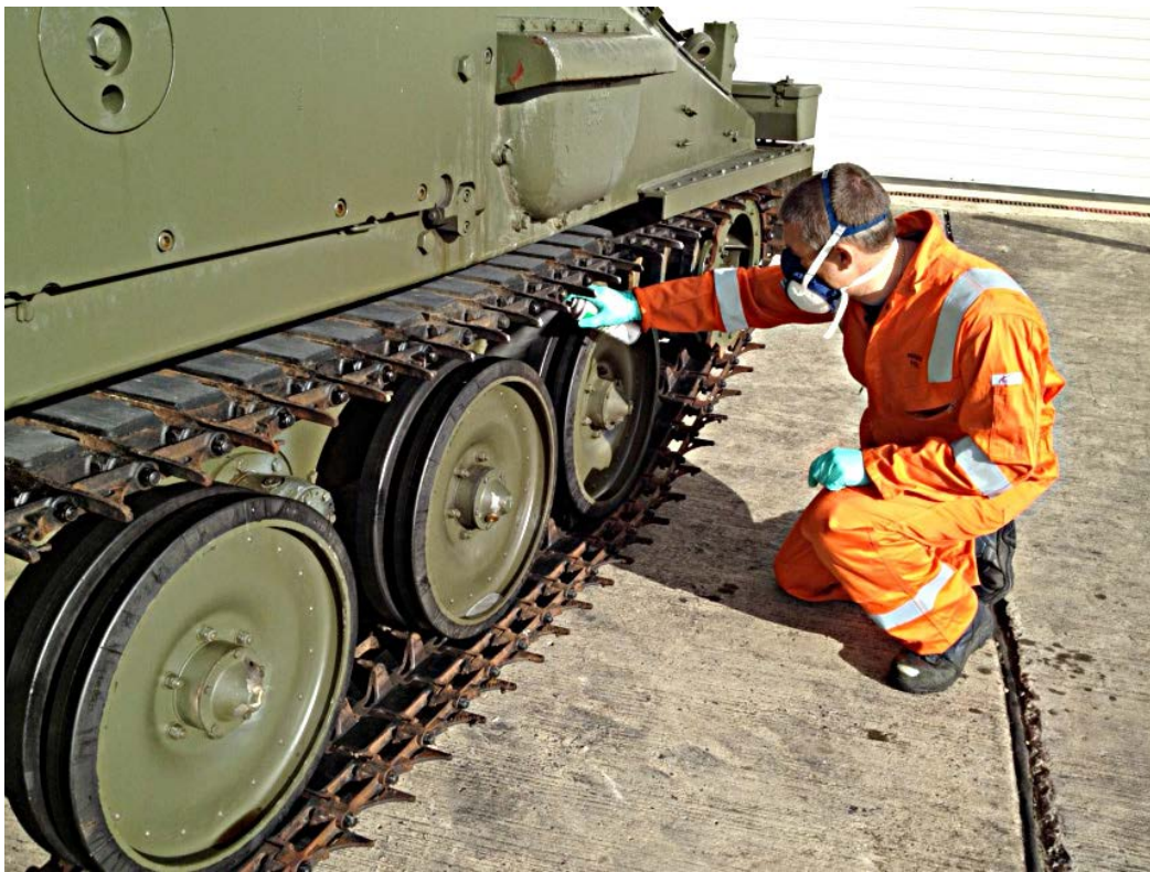
Figure 6: VCI aerosol used to protect Combat Vehicle Reconnaissance (CVR) (5) wheels. VCI additives were also used in the fuel, coolant, engine, gearbox, drive, and brake systems.
