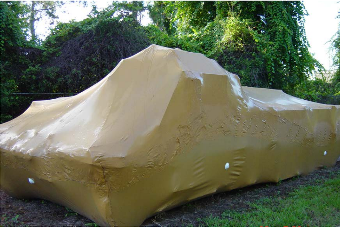
Figure 8: United States Air Force (6) Cargo Loader, preserved with VCI shrink film.
