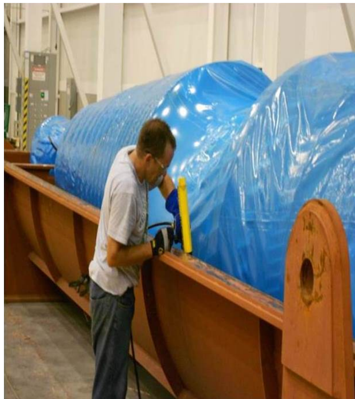
Figure 13: VCI shrink film being applied to rotor.
