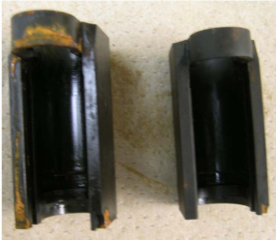
After 96 hours in ASTM B 117 Salt Spray. Castrol on left, VpCI-325 on right.
