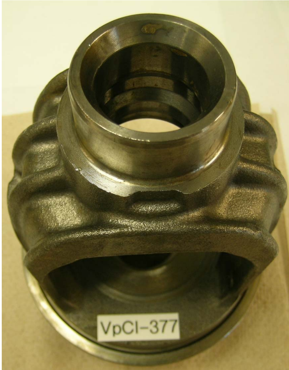
Part dipped in 5% VpCI-377, after 336 hours in ASTM D-1748 humidity cabinet.
