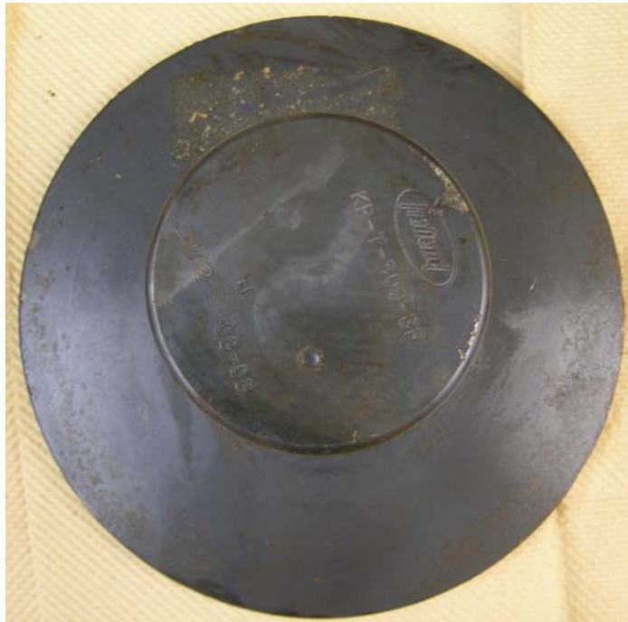
Figure 3: Part coated with VpCI-325, after 336 hours in humidity testing.
