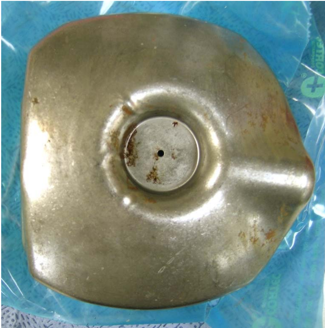
Figure 2: Metal stamping, wrapped in VpCI-126 blue film, after 840 hours of humidity testing.
