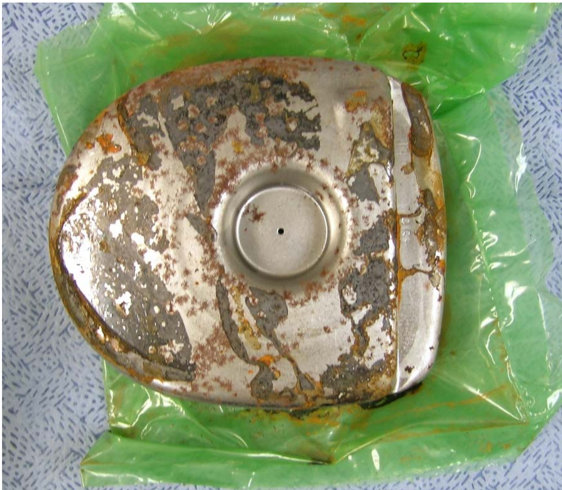
Figure 1: Metal stamping, wrapped in NTI film, after 840 hours of humidity testing.
