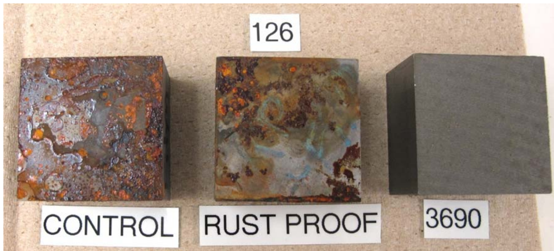
Figure 2: Blocks packaged in VpCI-126 film, after 576 hours of ASTM D-1735 testing.
