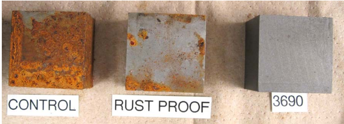
Figure 1: Blocks not packaged in VpCI-126, after 576 hours of ASTM D-1735 testing.
