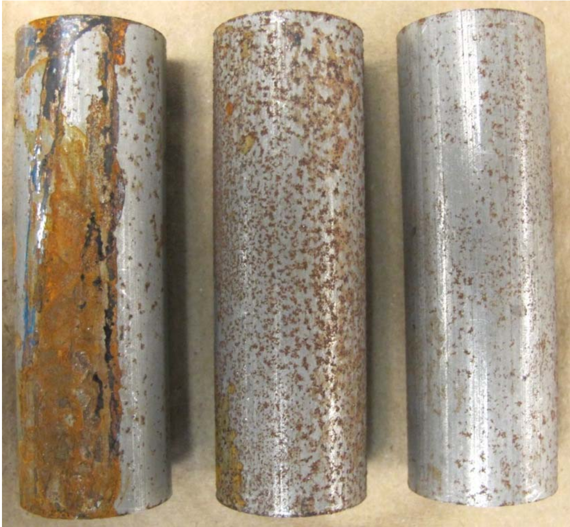
Figure 1: Tube sections after 168 hours of humidity testing. From left to right: Control, current cleaner, VpCI-416.
