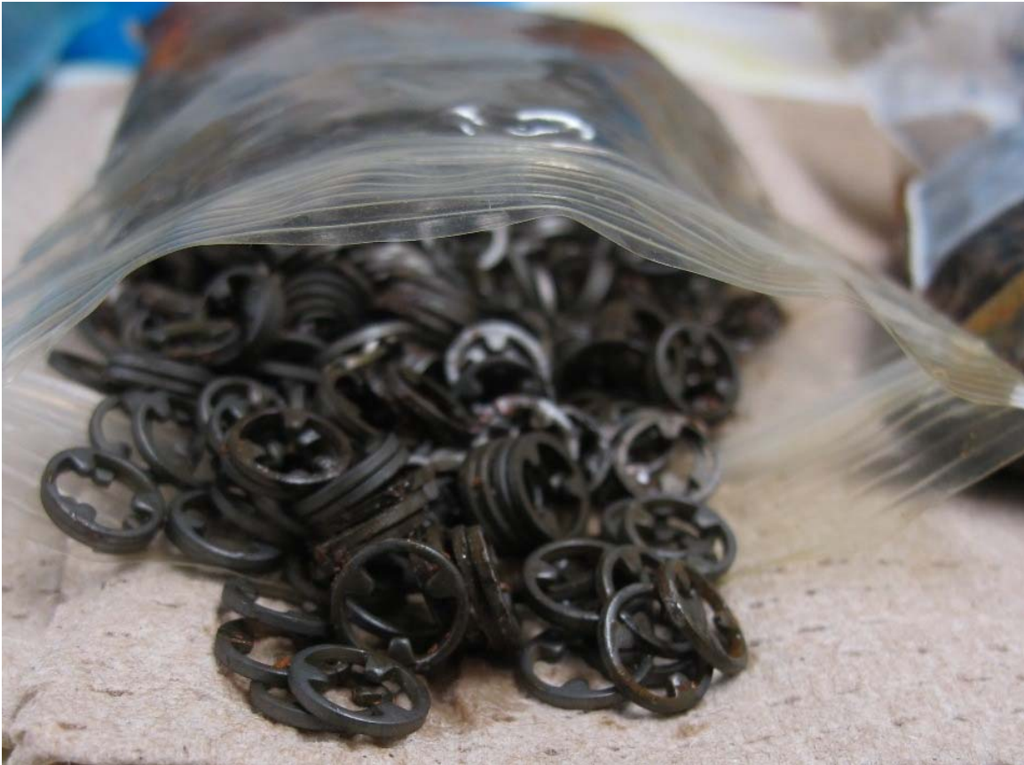
Figure 1: Untreated retainers after 840 hours of ASTM D-1748 testing.
