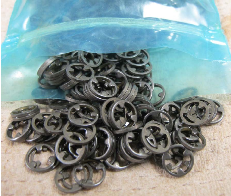
Figure 5: VpCI-126/416 parts after 840 hours of ASTM D-1748 testing.
