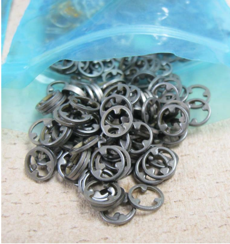
Figure 4: VpCI-126/337 treated retainers after 840 hours of ASTM D-1748 testing.
