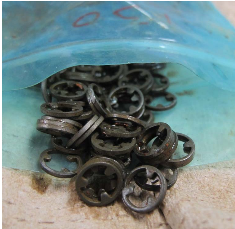
Figure 3: VpCI-126/133 retainers after 840 hours of ASTM D-1748 testing.
