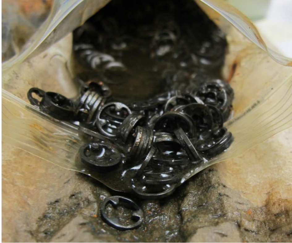
Figure 2: Rust Veto treated parts, after 840 hours in ASTM D-1748 testing.
