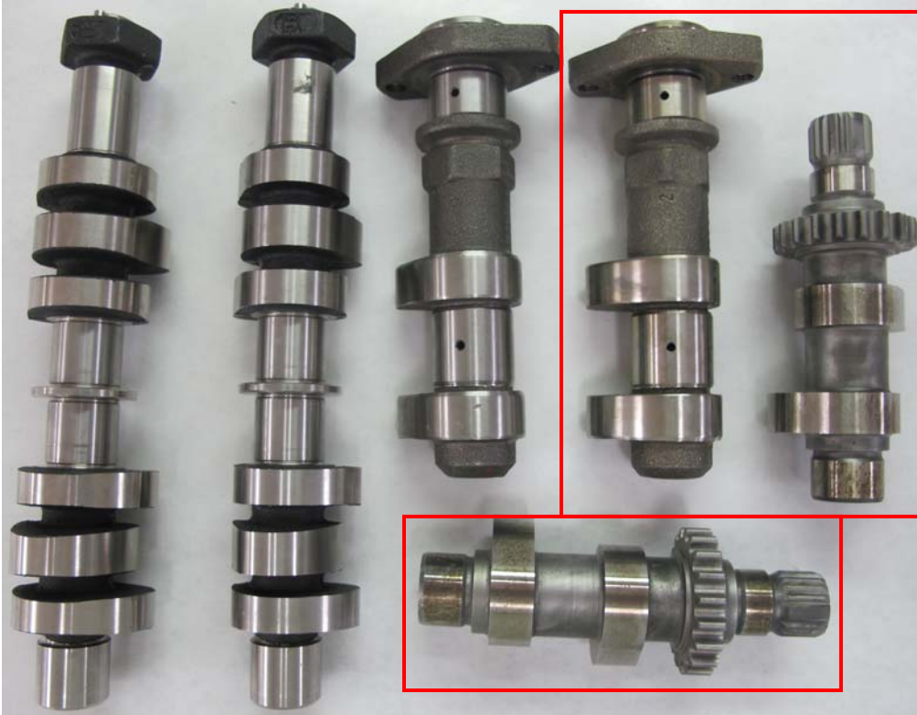
Three Parts after Rust Removal Highlighted in Red Boxes
