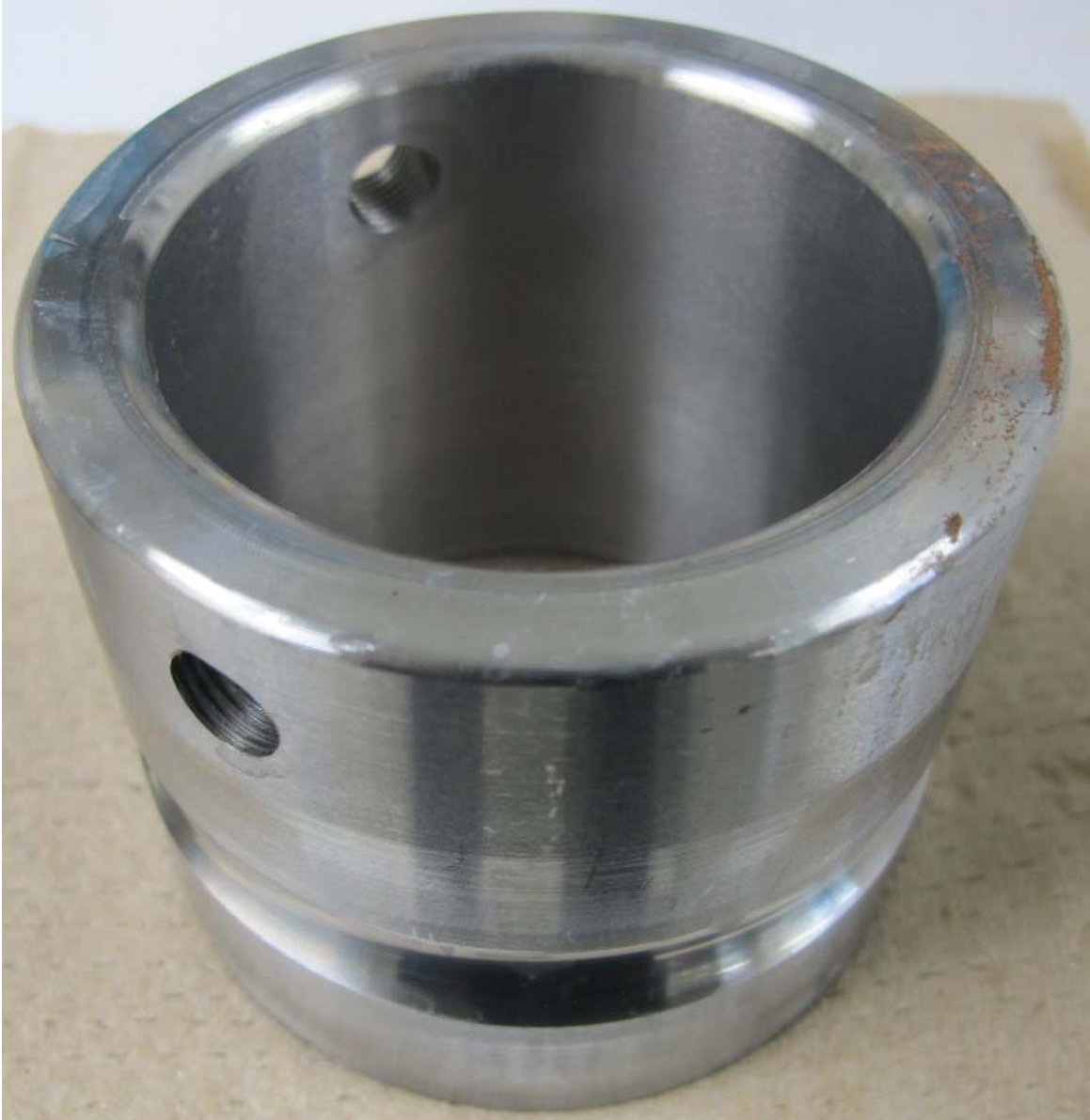
Figure 2: VpCI-126 packed part, after 504 hours in ASTM D-1735 testing.
