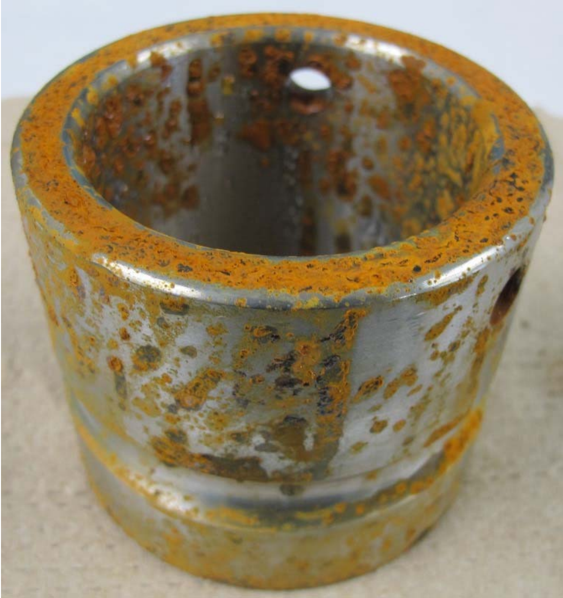
Figure 1: Non-VCI PE packed part, after 504 hours in ASTM D-1735 testing.
