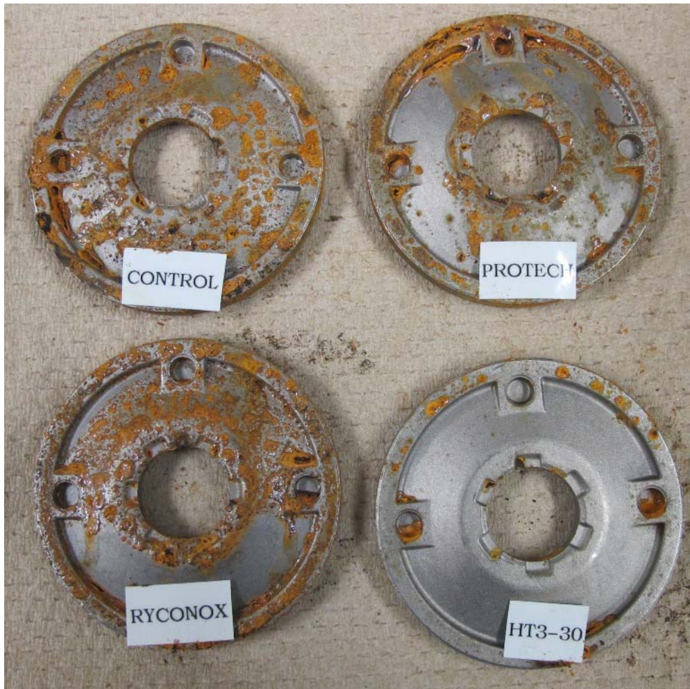
Figure 1: Four sintered metal rings, after 168 hours of ASTM D-1735 testing. The three rust preventives currently used by Customer were used in this group.
