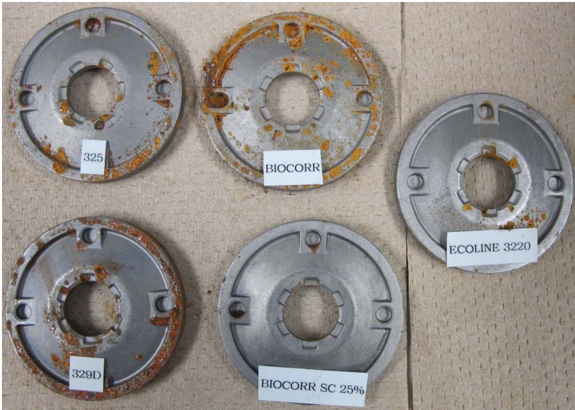
Figure 2: Five sintered metal rings, after 168 hours in ASTM D-1735 testing. The five Cortec rust preventive options were used in this group.
