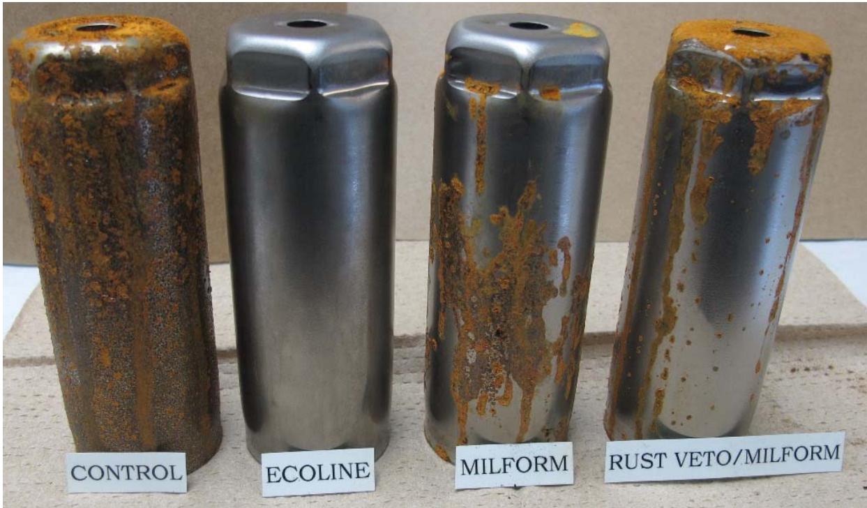
Figure 1: Customer's stampings after 144 hours in ASTM D-1735 testing.
