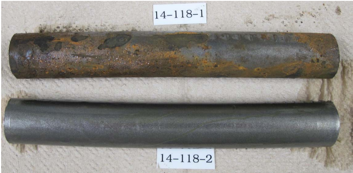
Figure 1: Capital Steel rods, after 504 hours in ASTM D-1735 testing. Condaprotect treated rod (14-118-1) and EcoLine 3690 treated rod (14-118-2).
