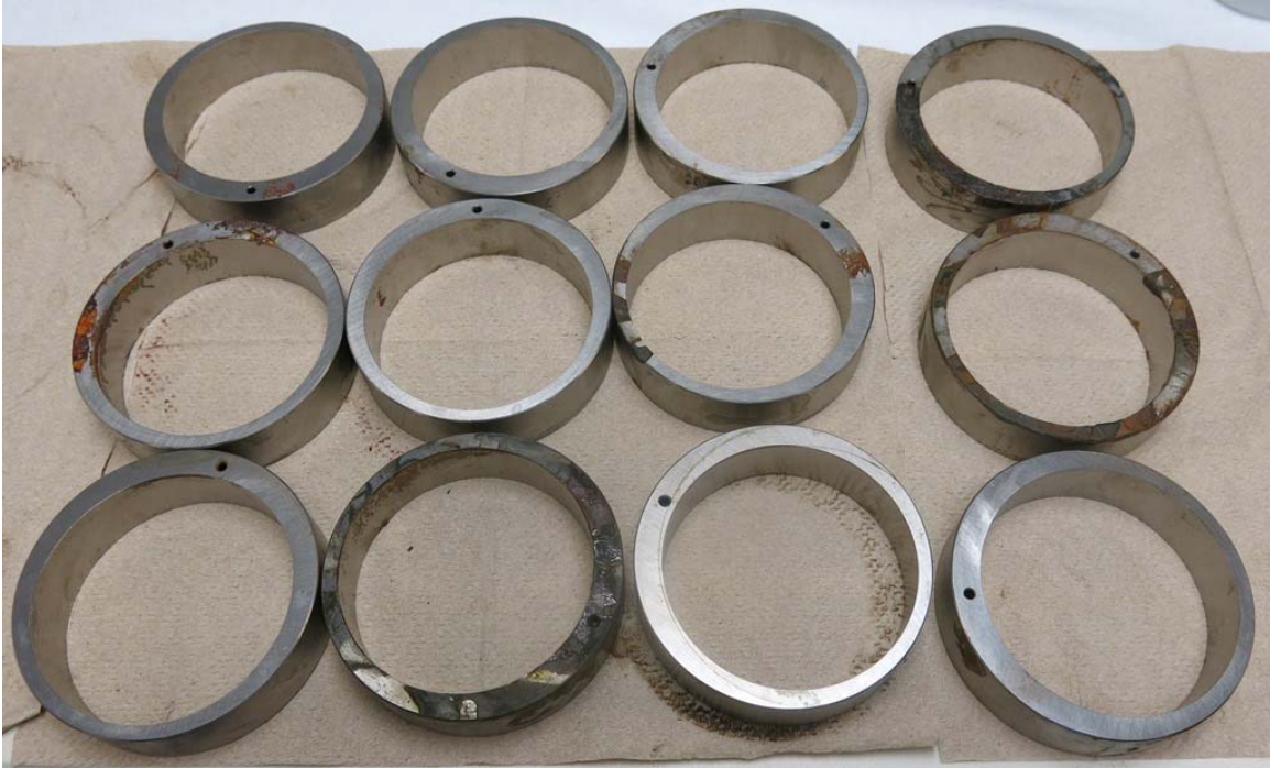
Figure 1: Zerust packaged parts, after 432 hours in ASTM D-1735 testing.
