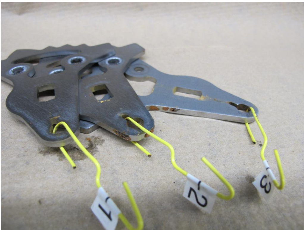
Picture 4: Condition of the Protech 1300 pieces after 9 days in the chamber
