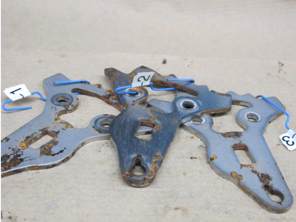
Picture 6: Condition of the Metkool pieces after 9 days in the chamber
