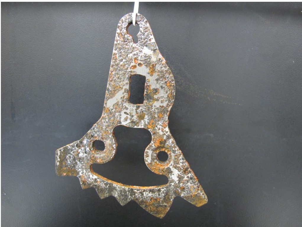
Picture 2: Condition of the control piece after less than 2 days in the chamber
