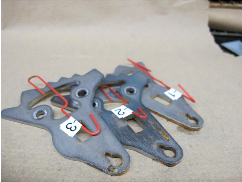
Picture 3: Condition of the VpCI-377 pieces after 9 days in the chamber
