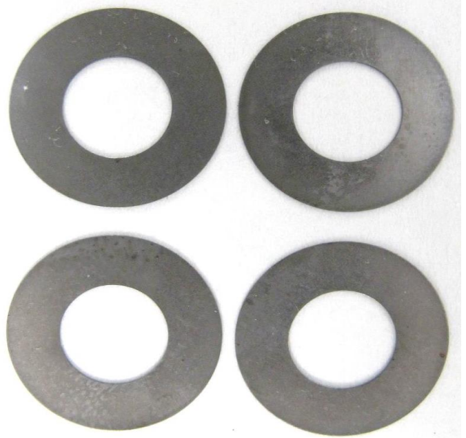
Sealed in VpCI-126 film with VpCI-130 foam
