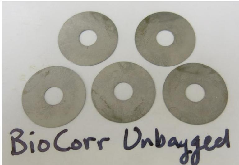
**Picture 2:** Washers protected with BioCorr Rust Preventative, left un-bagged in ASTM D-1748 conditions for 139 hour. Moderate discoloration can be seen on the washers.
