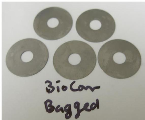
**Picture 5:** Washers coated in BioCorr Rust Preventative and bagged in VpCI-126 in ASTM D-1748 conditions for 139 hours. No discoloration can be seen on the washers.
