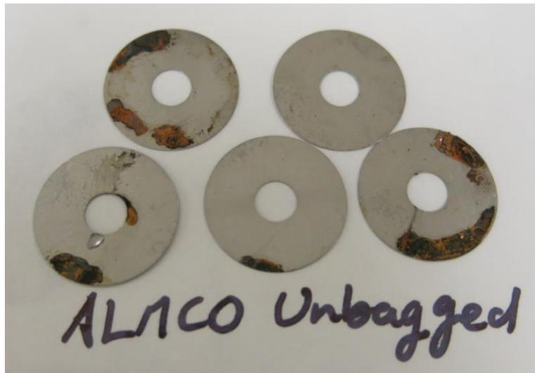
**Picture 1:** Washers protected with ALMCO 506R rust preventative, left un-bagged in ASTM D-1748 conditions for 139 hours. Severe rust can be seen on 4/5 washers.
