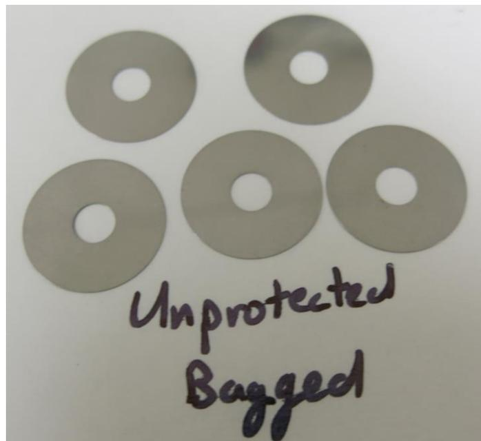
**Picture 3:** Washers, not coated with a rust preventative, bagged in VpCI-126 in ASTM D-1748 conditions for 139 hours. No discoloration can be seen on the washers.
