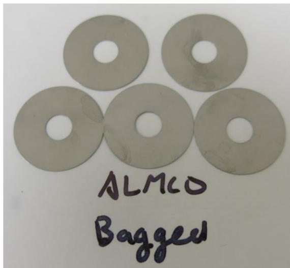
**Picture 4:** Washers coated in ALMCO 506R rust preventative and bagged in VpCI-126 in ASTM D-1748 conditions for 139 hours. No discoloration can be seen on the washers.
