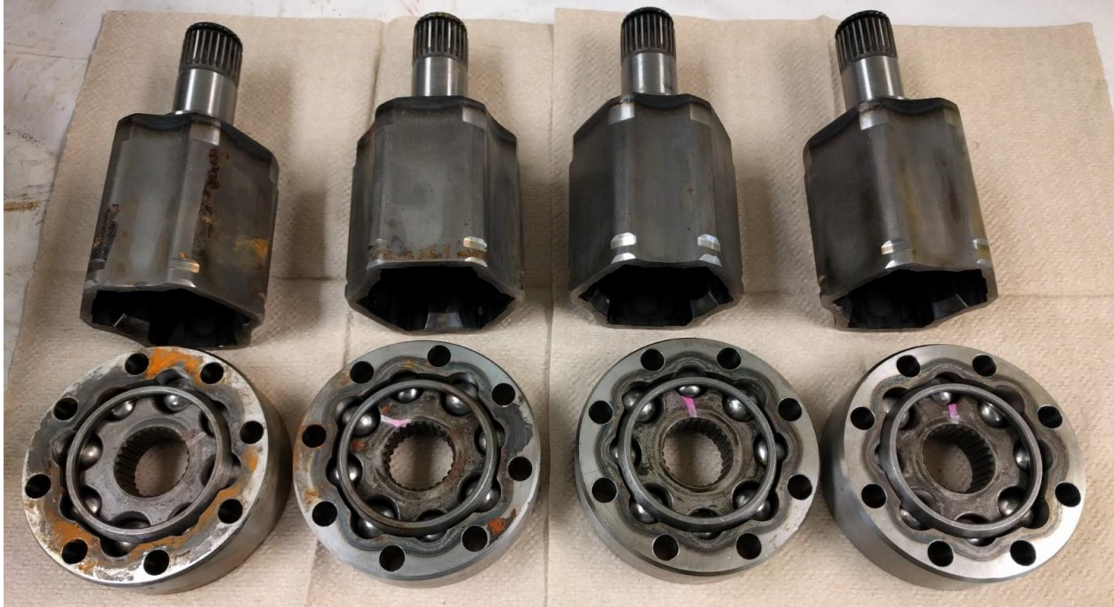
Figure 1: customer parts, after 600 hours in testing. From left to right: Control, Rustilo 4135HF, VpCI-325, EcoLine 3220.
