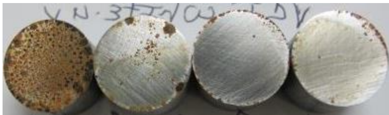
Figure 4: VCI White UV Film: Control, Plug #1, Plug #2, Plug #3 (from left to right).
