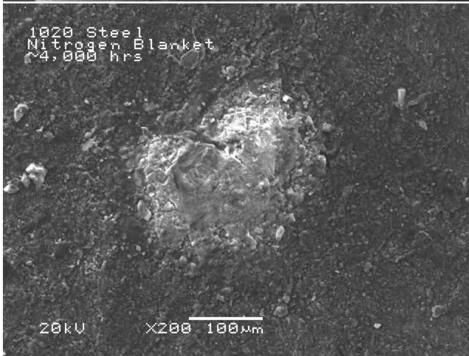
Figure 11: SEM micrographs of the LPR Probes (1020 steel) in nitrogen blanket protection system, show severe corrosion attacks on these sample surfaces. The thick red rust was removed to show severity of corrosion attack.
