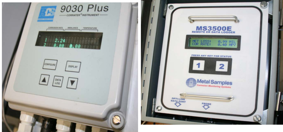
Figure 3: (left) RCS 9030 Plus Corratrator Instrument used for corrosion rate monitoring of 2 steel LPR probes (1 probe in 10% VpCI and 1 probe with nitrogen blanket); (right) Metal Samples MS3500E data logger used to monitor the corrosion rate for steel ER probes (1 probe in 10% VpCI and 1 probe with nitrogen blanket).
