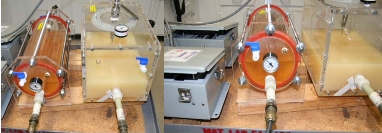
Figure 2: Test setup for corrosion test on steel LPR and ER probes using 10% VpCI or nitrogen blanketing at 10 psi applied pressure.
