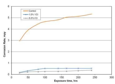
Corrosion behavior of steel pipes in boiling chloride water solution (200 ppm). Corrosion rate (mpy) of untreated control (orange) versus samples treated with 1% CorroLogic® CUI High-Temp Inhibitor (blue) and 5% CorroLogic® CUI High-Temp Inhibitor (gray).
