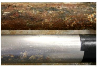
Pipe surfaces after 210 days of corrosion testing. CorroLogic® CUI Inhibitor was applied to the bottom pipe.
