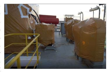
Shrink Film (extra heavy-duty) to get an external barrier with additional contact and vapor-phase protection.
