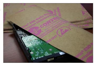
packaging paper for valuable electronic items. Vapor phase Corrosion Inhibitors (VCI/VpCI®) on one side of the paper form a protective molecular layer on metal surfaces wrapped inside, while another coating made from soybean oil dissipates static electricity buildup.
